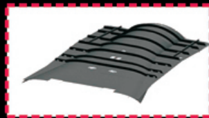
Trouser duct of center fuselage for LCA
