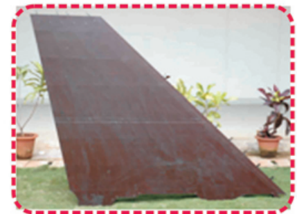
Co-cured Torsion Box for LCA Fin
