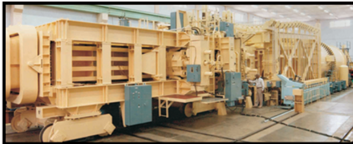
1.2 m trisonic wind tunnel
