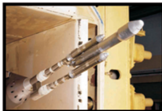
Twin sting support system for booster load measurements
