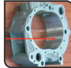
Ni-Sic coating deposited on the bore of the Trochoid housing of NAL's Wankel engine
