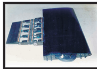
Smart aeroelastic wing model with an active control surface and an SMA-actuated rudder model.
