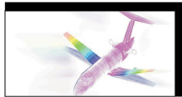
Full-aircraft finite element model of SARAS
