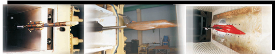
Clockwise: Aeroelastic testing of GSLV, SARAS T-tail and Tejas aircraft
