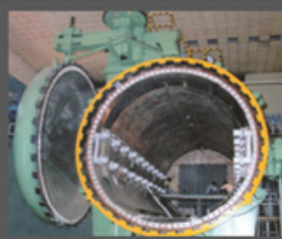
HAL 4mX8m – 2002 Working Space: 4m Dia x 8 m len; Max. Temp. 300°C Pressure: 10 barg
