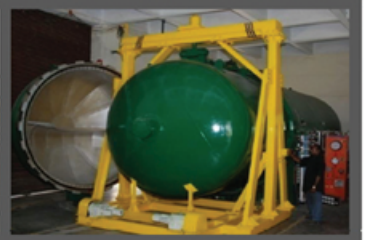
MARK II-1996 Working Space: 2.8 m Dia x 5.2 m Len Max. Temp. 250°C ; Pressure: 7 barg
