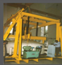
REAVES – 1999 (Revamped) Working space: 4.5m x 3.5 m height; Max. Temp: 200°C Pressure: 5 Barg
