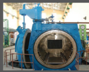
MARK III-2010 Working Space: 2m Dia x 4m Len. Max. Temp. 350°C and pressure: 15 Barg
