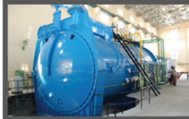
MARK IV-2009 Working Space: 4.4m Dia x 9m Len. Max. Temp. 250°C and pressure: 7 Barg
