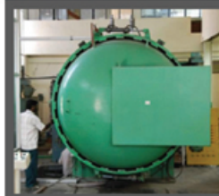
MARK I – 1986 Working Space: 1.8m Dia x 4m len; Max. Temp. 200°C Pressure: 7 barg
