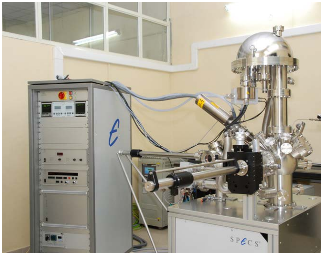
XPS System at SED-NAL
