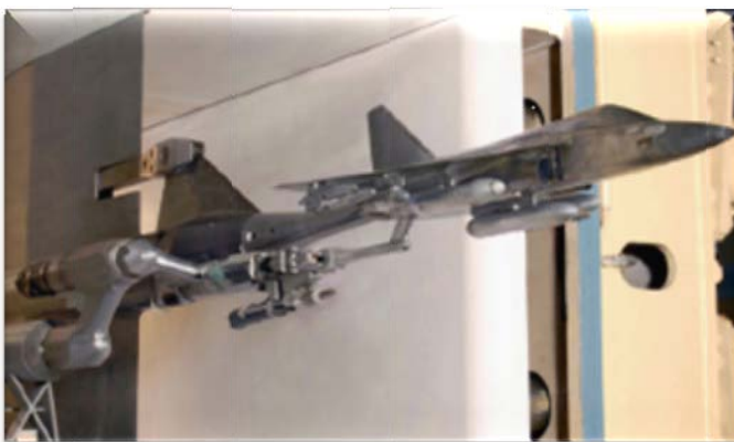
Captive Trajectory System for studies on stores separation from aircraft models
