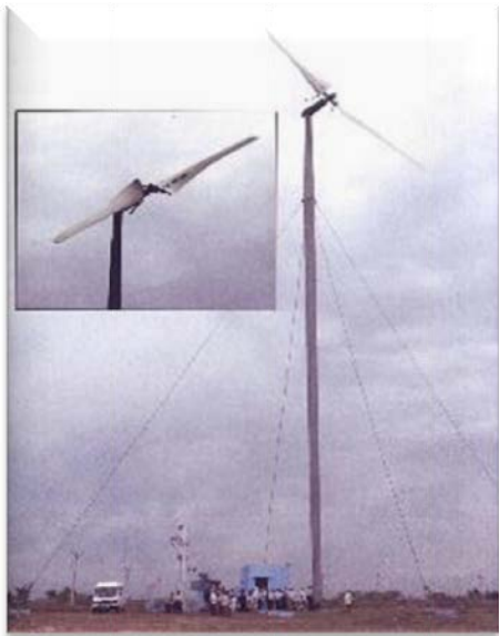
NAL-Sangeeth wind turbine blades being tested at Kethanur wind farm
